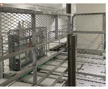
The cage inspection area allows stunned birds left in the cage after unloading to be removed manually.
